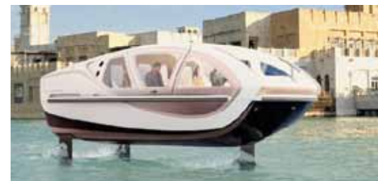
The sustainability-focused X-Pearl is powered by a hybrid hydrogen-electric propulsion system and retractable foils
